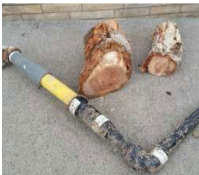
Old gas line "bandaid" and tree roots cut from trench
